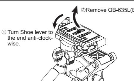
Turn Shoe lever to the end anti-clockwise. Then QB-635L(B) becomes loose. Remove it by sliding towards arrow.
