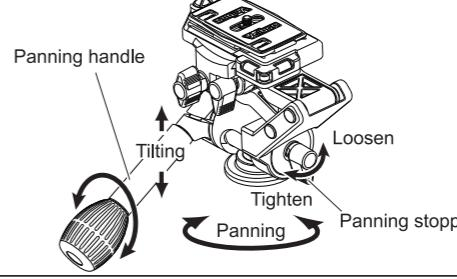
If rotating Panning stopper anti-clockwise, tilting is possible. If loosening Panning stopper, panning is possible.
