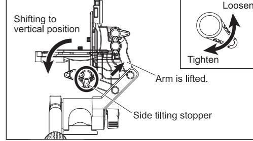
Vertical position is obtained firstly by loosening Side tilting stopper, and secondly by raising Arm while laying camera towards left. Afterwards tighten Side tilting stopper firmly. When the form is decided, tighten each stopper firmly and release the shutter.
