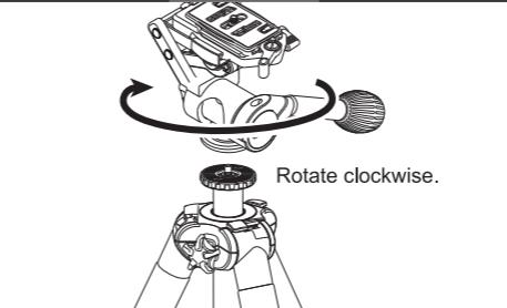
In order to install PHD-66Q to tripod, firstly tighten all the stoppers of PHD-66Q and tripod including Elevator stopper. Align Tripod screw of PHD-66Q with Camera screw of tripod, and rotate PHD-66Q clockwise as shown firmly.
