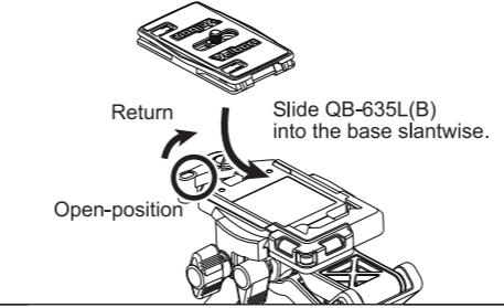
Firstly, slide QB-635L(B) into the base and push it downward. Then Shoe lever returns automatically as shown. While Shoe lever is in open-position, slide QB-635L(B) into the base from the side of Shoe lever slantwise. Then push it downward. Shoe lever turns automatically. Afterwards, push Shoe lever to the end clockwise manually.
