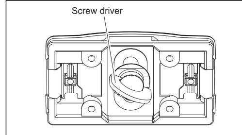
Align Camera screw into the hole of camera. Turn Camera screw clockwise by Screw driver attached firmly.
