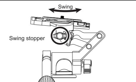
When adjusting Camera plate for horizontal position, firstly loosen Swing stopper and slide Camera plate from side to side.
