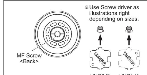
When purchasing, the size of Tripod screw is UNC1/4. If you want the size of UNC3/8, change MF Screw by using Screw drivers attached or coin.
